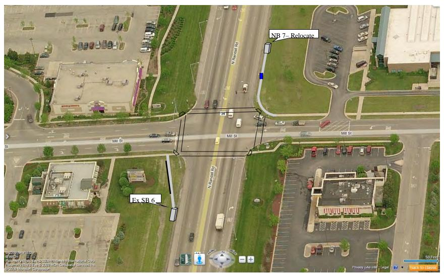
Tier 1: Relocate existing bus stops NB and SB to meet Pace Bus Stop Location Guidelines, construct bus shelters, add crosswalks and access ramps at all 4 corners of the intersection. Due to steep ditch at SW quadrant, recommend walkway be retained to cross over ditch.
