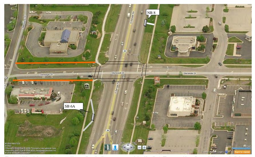
Tier 1: Add bus shelter to existing stops, add crosswalks and walkway to connect to existing sidewalk. At SB stop, transition walkway to bridge over exist ditch.
