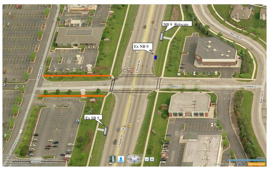
Tier 1: Relocate existing NB 9 stop, add bus shelter, add crosswalks and add walkway to connect to existing sidewalk. Add Bus shelter to existing SB 5 stop. Tier 2: Add sidewalks in NW and SW quadrant to connect to existing sidewalks.
