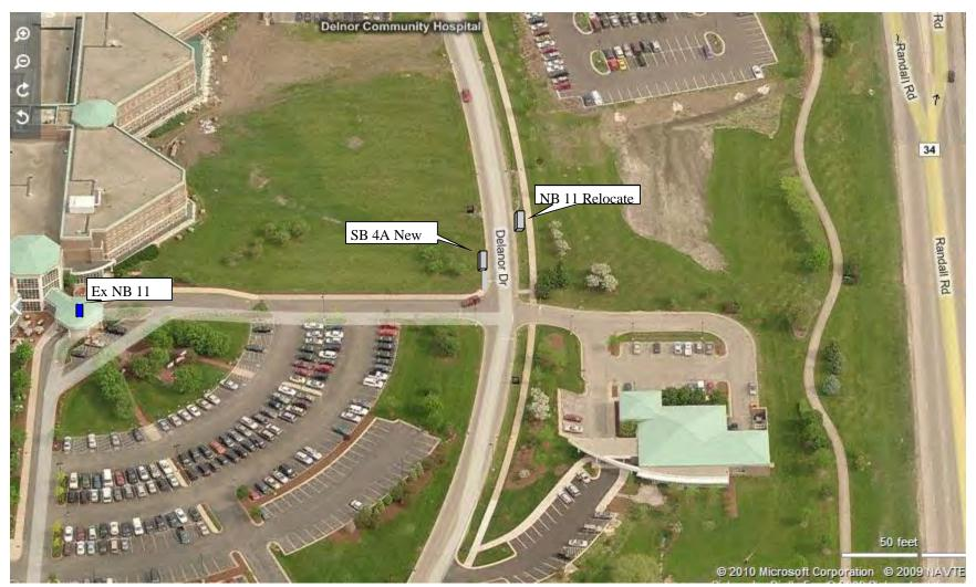
Tier 1: Relocate Existing NB11 stop to Delnor Dr, Add bus shelters and add sidewalk where required to connect to existing sidewalk.
