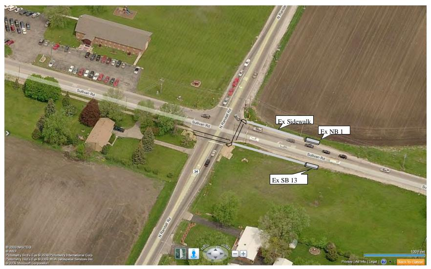
Tier 1: Maintain location of existing NB and SB stops, add bus shelters, add sidewalks, crosswalks, and access ramps. Tier 2: No proposed improvement at this time.
