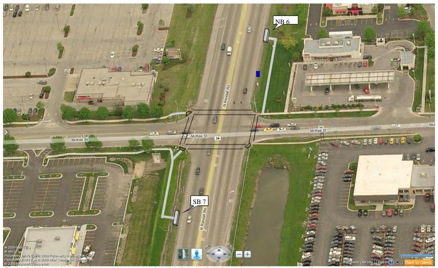
Tier 1—Build bus shelters and relocate exist stops to meet Pace Stop Location Guidelines, add crosswalks, construct walkway to connect to existing sidewalks. AT SB 7, there exists a big slope and ditch, culvert may be extended or build sidewalk to bridge over ditch area Tier 2—No Improvements proposed.
