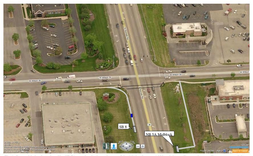
Tier 1: Due to right hand turn lane, New NB 5A stop placed prior to the start of the right hand turn. Add bus shelter, walkway and crosswalk to connect to existing sidewalks. Relocate existing SB8 to meet Pace standards and add walkway to connect to existing sidewalks.
