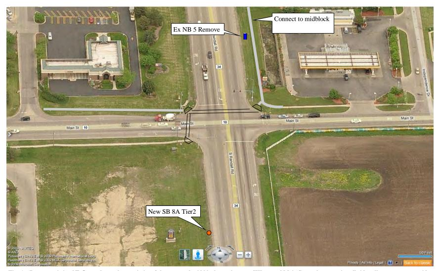
Tier 1—Remove existing NB 5 stop due to the proximity of the proposed mid block stop between Wilson and Main Street, however, install sidewalks to connect to mid block stop, add sidewalk, crosswalk and access ramps north of Main St.
