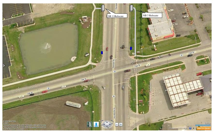
Tier 1: Existing Stops are too close to intersection—relocate to the north in accordance to Pace Standards, add sidewalks at the NE quadrant to connect to existing sidewalks
