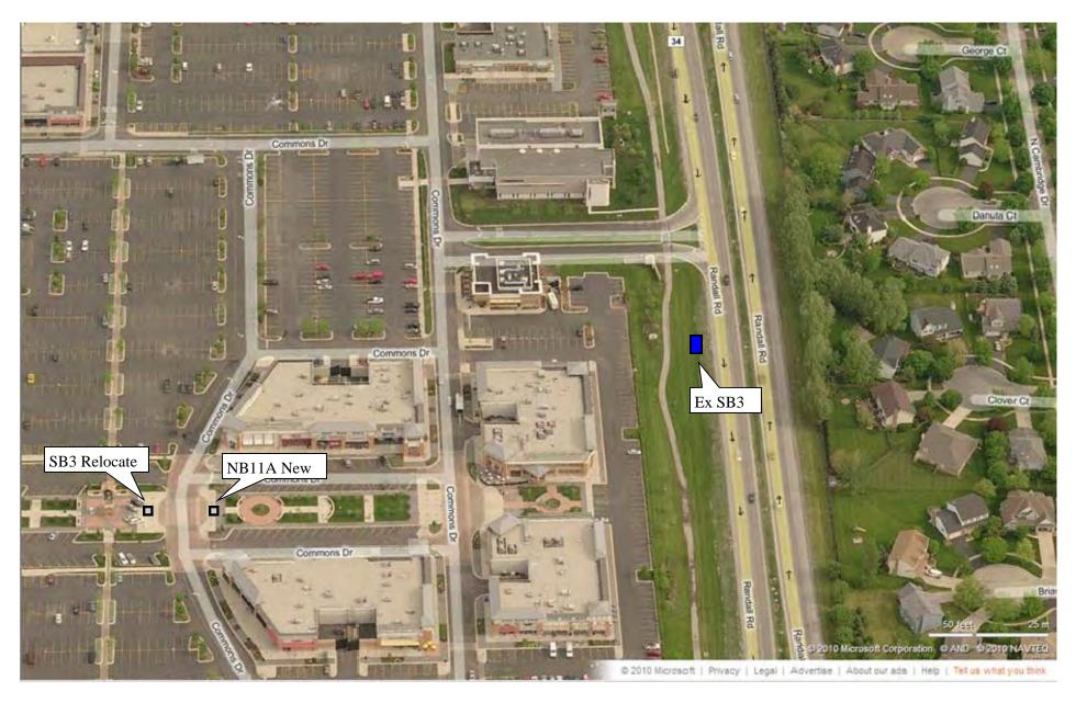
Tier 1: Move Existing SB 3 stop inside Geneva Commons. Install a sign on a post. Add NB 11A stop.
